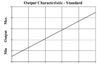
Retracted Linear Displacement Extended
